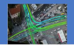
On the right are illustrated the trajectories of any single traffic light phase. Was created a filter that visualizes the trajectories of specific entry and exit Gates, for any image we can see the possible manoeuvres of any traffic light phase; obviously the manoeuvres were made in different times during the analysed interval (30 minutes, from 7:45 A.M. to 8:15 A.M.).
